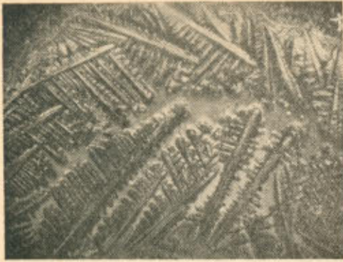
Fig. 1 Total typical crystallisation—x 250.
